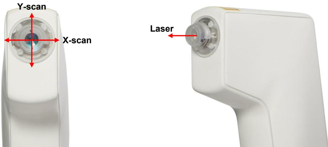
The topical probe has been designed to be held comfortably in either the left or right hand, and operates in any orientation for ease-of-access to the region being imaged. It incorporates a colour camera (with white LED illumination) which shows on-screen the area of skin being imaged and the exact location of the scan line, to assist the user with positioning the scan on the area of interest.
