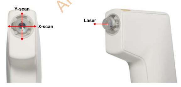
The topical probe has been designed to be held comfortably in either the left or right hand, and operates in any orientation for ease-of-access to the region being imaged. It incorporates a colour camera (with white LED illumination) which shows on-screen the area of skin being imaged and the exact location of the scan line, to assist the user with positioning the scan on the area of interest.
